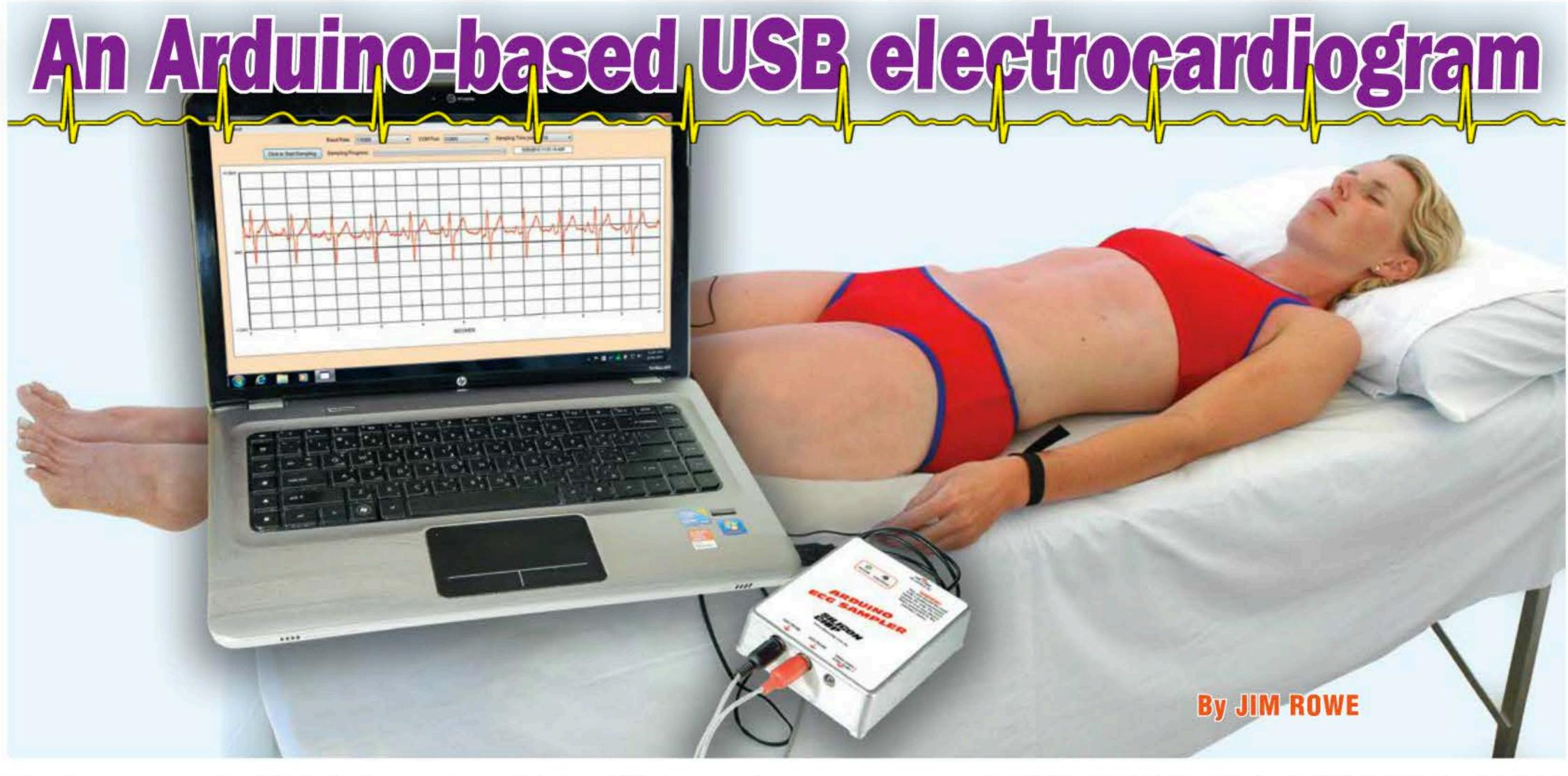
Here's an easy-to-build Arduino project which will let you take your own electrocardiogram (ECG) and display it on a laptop PC. The software lets you read, display, save and print the electrical waveform generated by your heart – or anyone else's. It connects to your laptop via a USB cable, which also provides the low power it needs to operate.
