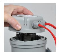
process can prove quite difficult when at the top of a ladder. The One-Shot horn eliminates screw removal by utilising a patented twist lock mechanism. The installer simply twists off the rear cover, connects the cabling and twists the cover back on. The labor savings by using the One-Shot horn on a large job are significant. To further cut installation time, a patented 'dog leg' mounting bracket is employed which eliminates the need to separate the horn from the bracket during installation.
