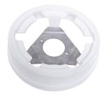
The C 0699A adaptor plate enables the speaker mounting rings to be fixed to a standard recessed conduit junction box without the need for drilling into the concrete slab, saving considerable installation time & hardware.
