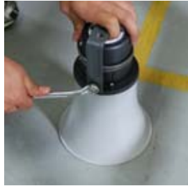
Step 1 Remove bracket from horn speaker.
