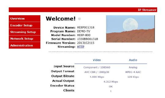
On the Welcome Screen, we have added a tool to help the installer locate a unit in a rack or headend. Press the LED ON button (shown below). This will cause the CFG LED light to flash continuously for the installer to identify and locate the HDIP. To turn off, simply press the LED tool again.
