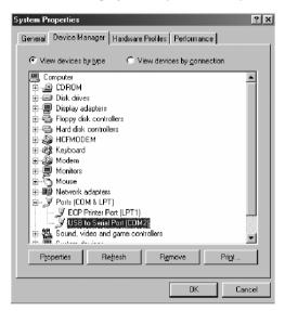
When the driver is installed properly, "USB to Serial Port" will appear on the Device Manager.
