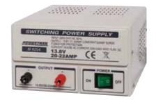
A fixed voltage output power supply designed for powering automotive, marine and comms equipment. Low noise and ripple design (<100mV) offers excellent efficiency and performance for the electronics work bench. Size: 210W x 130H x 260Dmm. Weight: 1.5kg.
